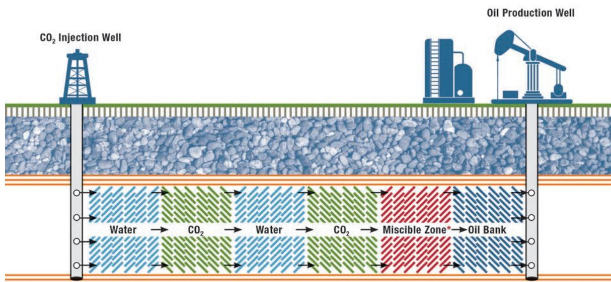
\*Miscible Zone = Injected CO<sub>2</sub> encounters trapped oil → CO<sub>2</sub> and oil mix → Oil expands and moves towards producing well
