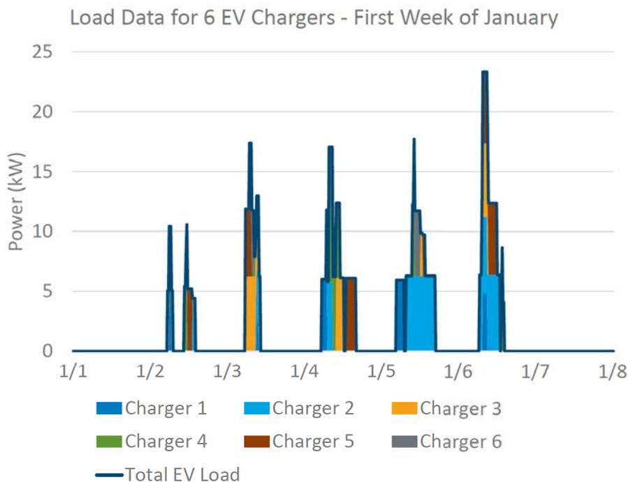
Source: Elgqvist et al (2019). This figure shows six chargers for a week in January. The charging profiles were developed for this project, incorporating winter and summer charging profiles that reflect temperature data for Minneapolis, Minnesota
