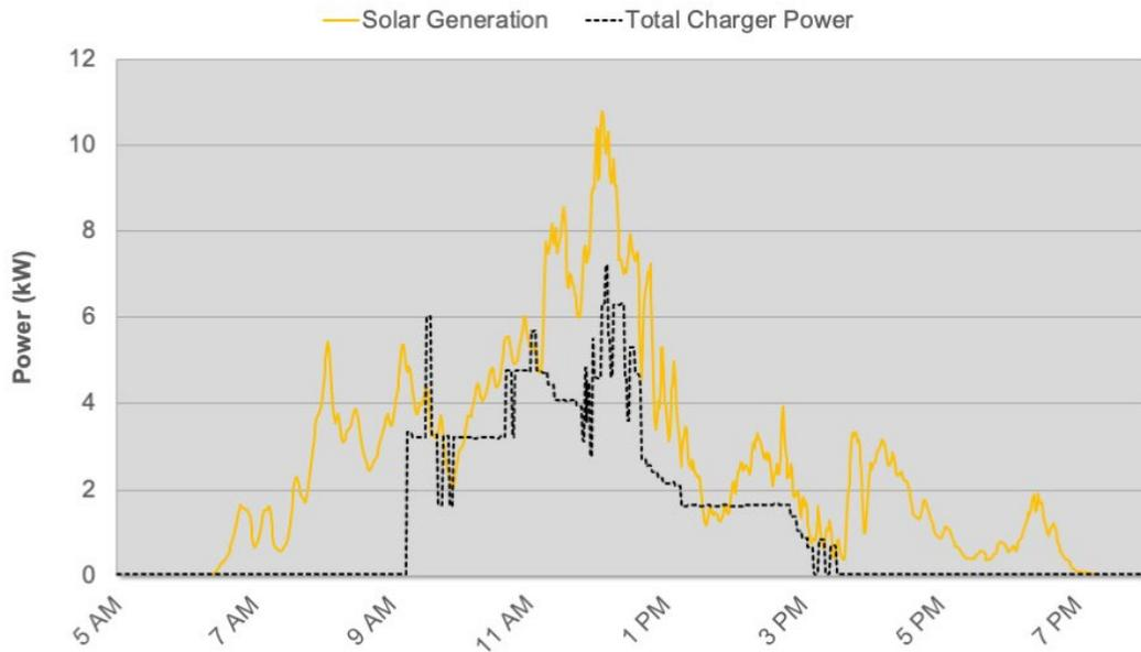
Source: GPI analysis. A mostly cloudy day with intermittent solar production. Some mismatch of charging is shown because the charging data is shown at five-minute intervals and the solar production is at one minute.
