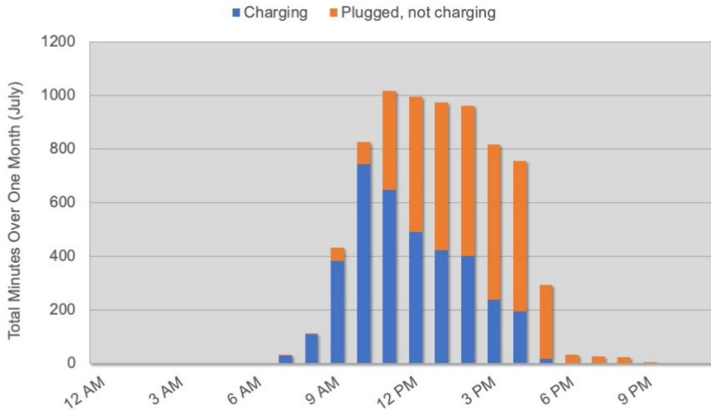
Source: GPI analysis of Greenway pilot project. Vehicles are getting fully charged early in the day, as July sun is sufficient in the morning to meet charging demand. Vehicles are generally plugged in far longer than needed to charge.
