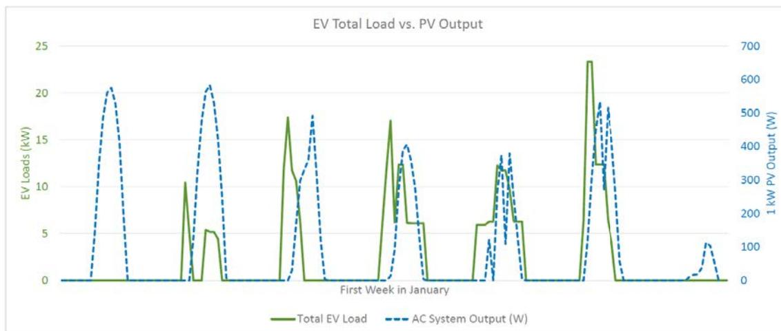
Source: NREL analysis for Minnesota SEIN project, showing the modeled charging patterns for six workplace chargers and the solar production curve for a January week. The timing mismatch is broadly consistent across days but could be matched through managed charging with a shift of only a couple of hours.
