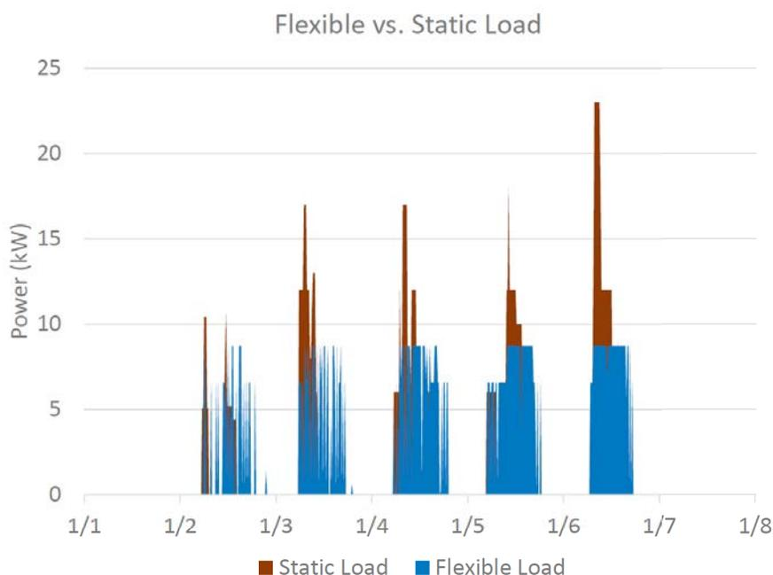
Source: NREL analysis conducted for the Minnesota SEIN project. This chart superimposes unmanaged charging (red) and managed charging (blue) to avoid simultaneous peaks from individual EVs for six chargers being used during the day at a workplace or public parking facility where cars are parked for most of the business day. The peaks from the six chargers in the unmanaged scenario also sometimes coincided with building load peaks.
