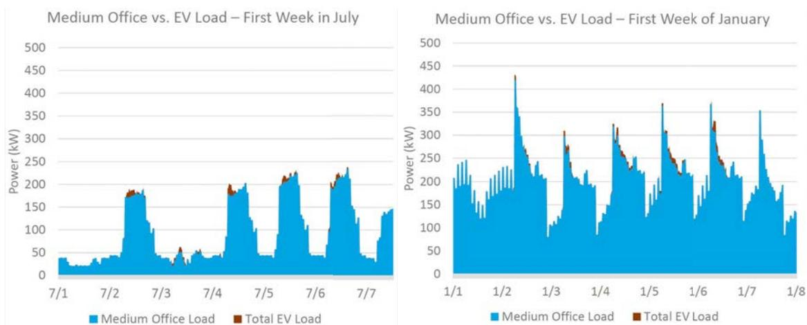
Source: Elqvist et al (2019). Demand from six EV chargers is quite small compared to this building load, but still contributes to peak demand on most days, in both July and January. The building electric load profile for a mid-sized office building in an urban Minnesota location is based on DOE's reference buildings.
