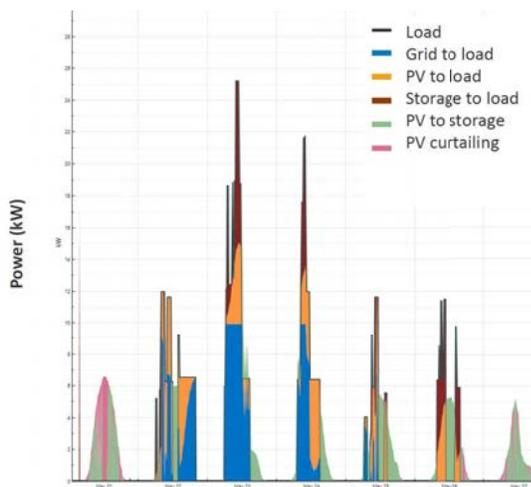
Source: NREL REopt analysis. The solar array directly supplies the charger, charges the battery, or is curtailed (no credit is modeled for net metering).
