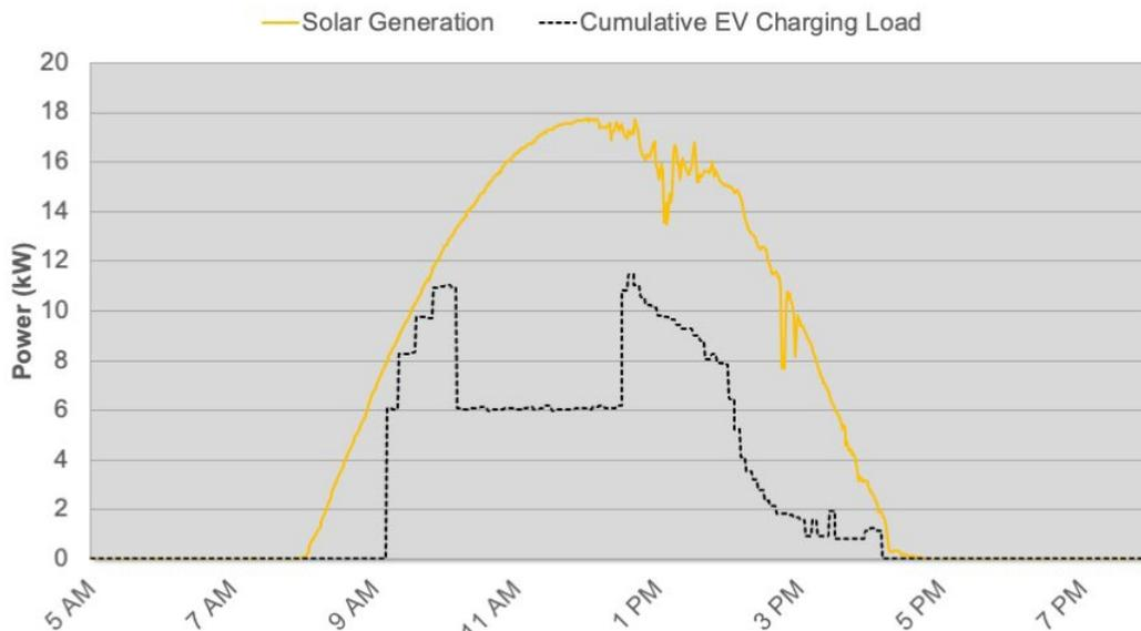
Source: GPI analysis of the Greenway solar synchronization pilot project. On this January day, solar production does not ramp up until after the start of business hours and declines prior to the end of business hours. In this case, no more than two chargers were used at any one time, and only one brief moment of simultaneous charging. Chargers will provide at least a Level 1 charge, regardless of solar production.
