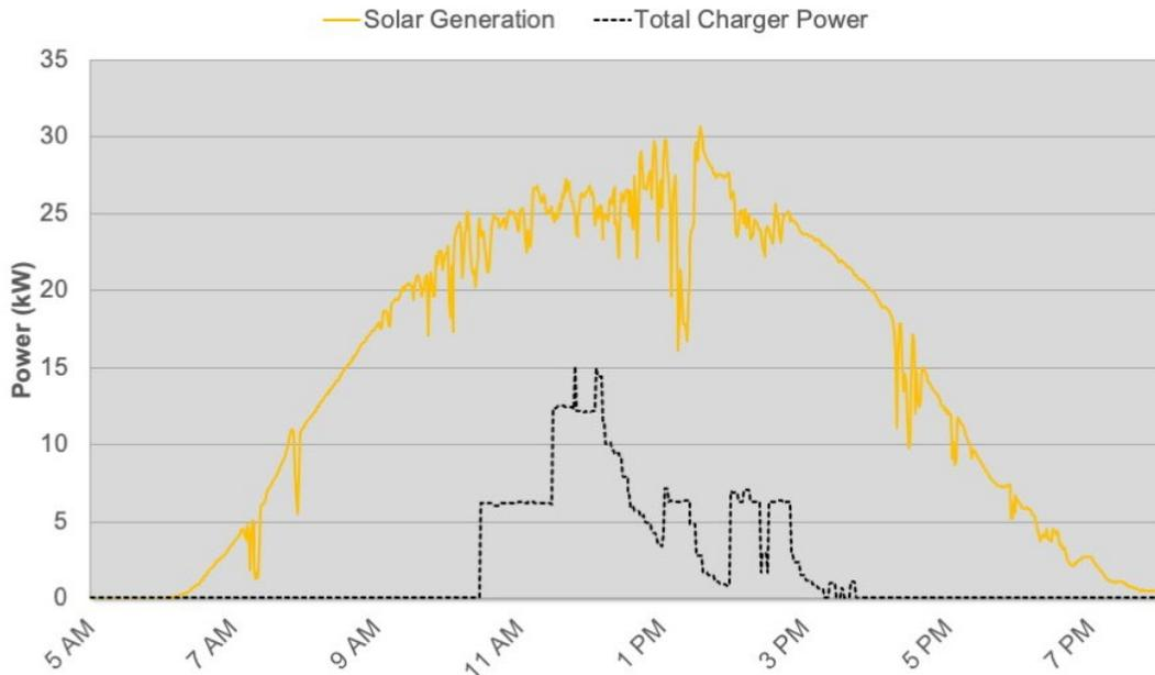
Source: GPI analysis. Solar production (late July) substantially exceeds maximum EV load. Even at 9:00 a.m., the solar capacity would cover the 15 kW peak. In contrast, winter solar production and cloudy days present circumstances when synchronized charging is needed to reduce demand charge impacts.
