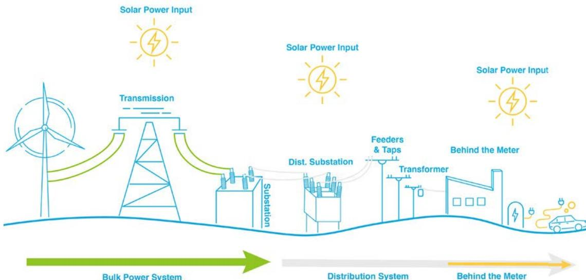
Source: GPI. Solar+EV value can be captured at any or all of the three segments, and EV charging can be synchronized with solar inputs at each of the value segments. Because EV-charging is always a distributed energy resource, value from solar+EV applications can move upstream to create value (e.g. behind the meter synchronization can provide some benefit or value in the bulk power system).
