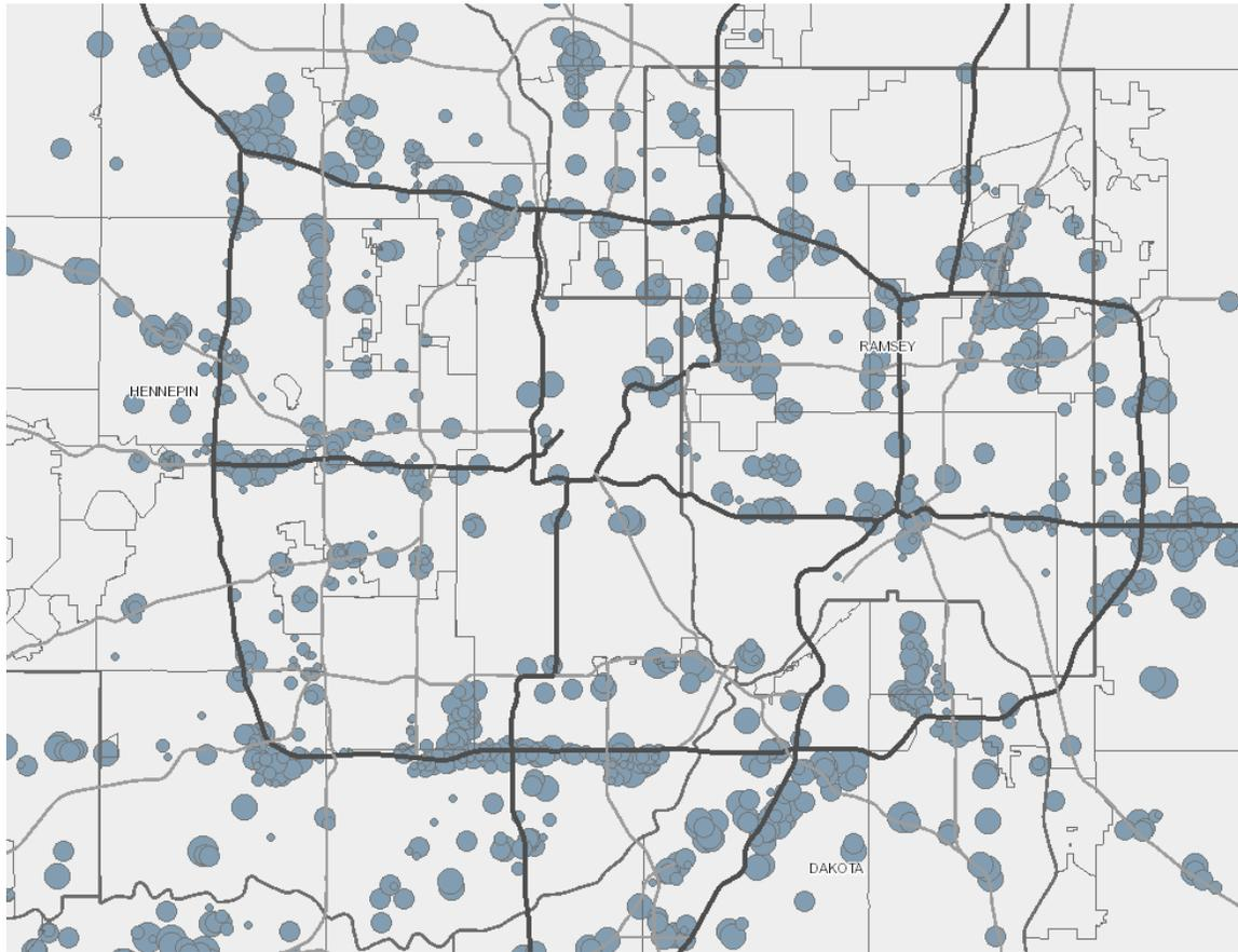
Source: Metropolitan Council GIS Map viewer. The size of the circle indicates the solar development potential for this site. Most of the circles show solar potential over a MW in size.
